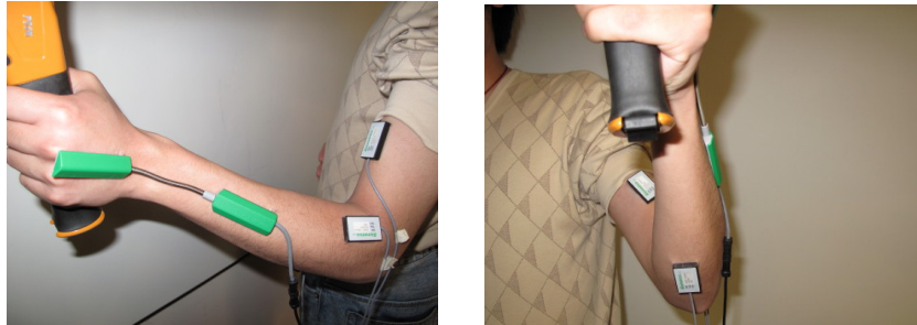
Figure 3 Placement of surface electrodes and goniometer
